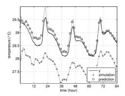
Fig. 4. Temperature y measured by one internal sensor not included in the output set  $\mathcal{L}$  vs.  $y_u$  simulated using the PBSID<sub>opt</sub> model and  $\hat{y}$  predicted by the Kalman filter using 5 outputs in the set  $\mathcal{L}$ .
