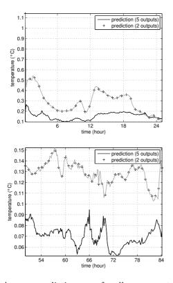
Fig. 6. Average prediction error for all sensors not included in the set  $\mathcal{L}$  during transient period (top) and at steady-state (*bottom*). Predicted output  $\hat{y}(t)$  using the Kalman filter with 2 and 5 outputs.
