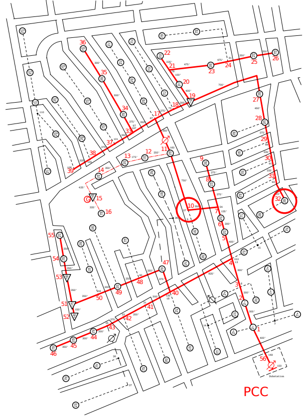
Fig. 3. The IEEE 123-bus test feeder. In red, the three-phase backbone that has been considered in the simulations, as detailed in [28]. The distribution feeder is connected to the MV network at the PCC. Two nodes (circled in red) host a microgenerator each, both capable also of injecting reactive power in order to support the feeder voltage profile.
