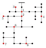
Fig. 2. Schematic representation of the IEEE 37-bus test feeder. Red nodes represent prosumers behaving as generators, as their power generation capability exceed their power requirement. Black nodes instead represent prosumer behaving as loads, whose power demand is bigger than their generation capabilities.
