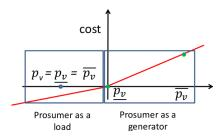
Fig. 1. Power cost function associated with a prosumer.
