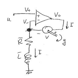
$$V_{\circ} = A(V_{+} - V_{-})$$
