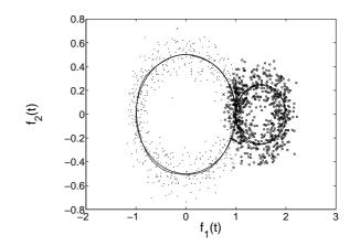
Fig. 2. Robot's path reconstruction. True path f (thick line), noisy measurements (points, circles and x-marks) and estimate of f using periodic cubic smoothing splines (thin line)
