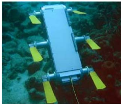
Figure 1.6: The hexapod underwater robot AQUA .
