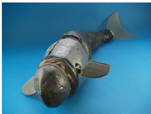
Figure 2.2: RoboSalmon V2.0 vehicle with Tendon drive tail attached.
