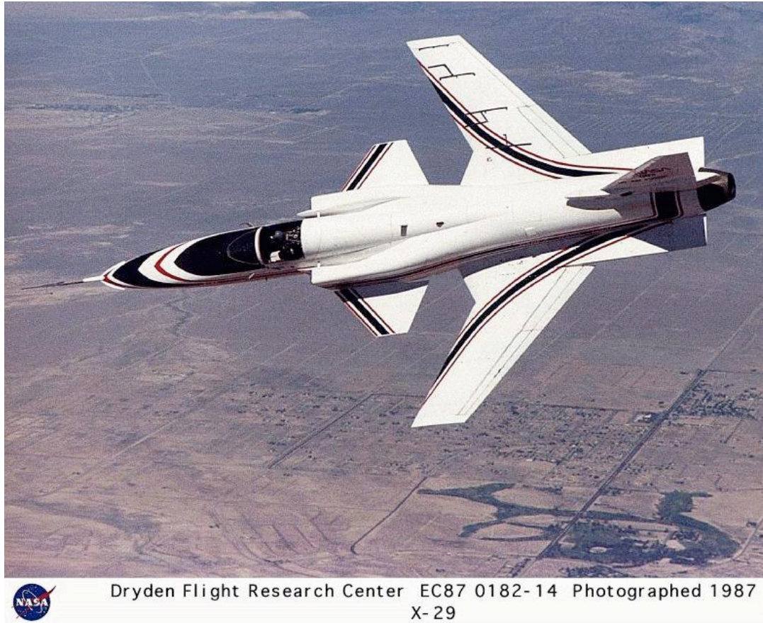
FIGURE 1.4: Nasa x-29 forward swept wing aircraft. Its dynamic instability makes it highly maneuverable, even though a closed loop control is required to be constantly active.
