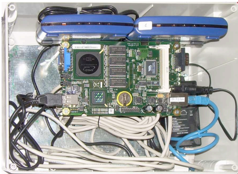
Figure 2. An example of Node Cluster Gateway (NCG), showing the embedded computer in the center, and the two USB 2.0-compliant hubs at the top.
