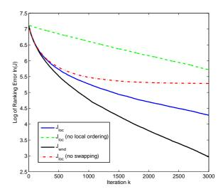
Fig. 3. Average (over 100 Monte Carlo runs) of the ranking error of Algorithm 2 in a random geometric graph with 50 nodes and 250 edges.
