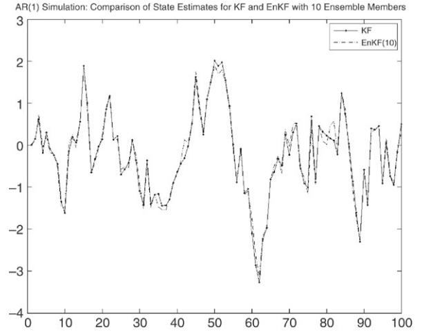
Fig. 6. First-order autoregressive process simulation Kalman filter state estimates and EnKF filter state estimates based on 10 ensemble members.
