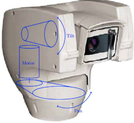
Fig. 3. Positioning unit for surveillance cameras.
