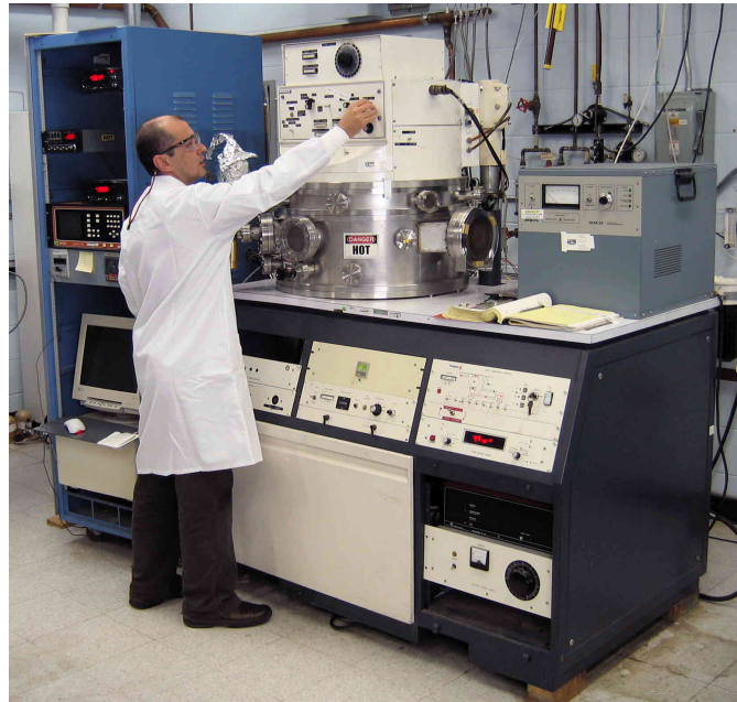
Figure 5.1: A Plasma for Chemical-Vapor Deposition. Photo courtesy of Argonne National Laboratory http://www.anl.gov/
