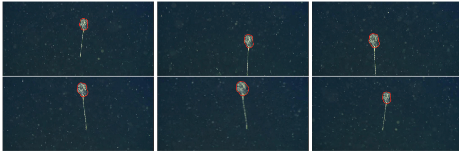
Figure 3.7: Sea Flower image sequence Active Contours are unreliable on blurry images such as underwater shots, where camera movements and the diffusion of the light make edges dull. Generalized Active Contour provides a better shape detection tool, in this case easily embedding the color information
