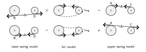
Each sub-model has only one fully linear (bilateral) spring and holds when it is tense.
