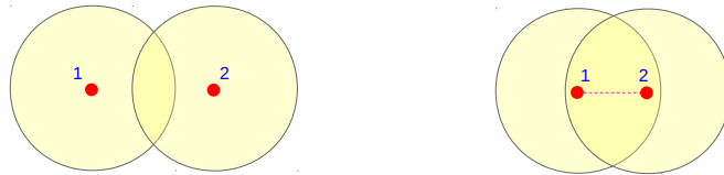
Figure 3.8. Visibility radii determine whether two agents are neighbors (right) or not (left). Image taken from Ramaithitima et al. (2015).
