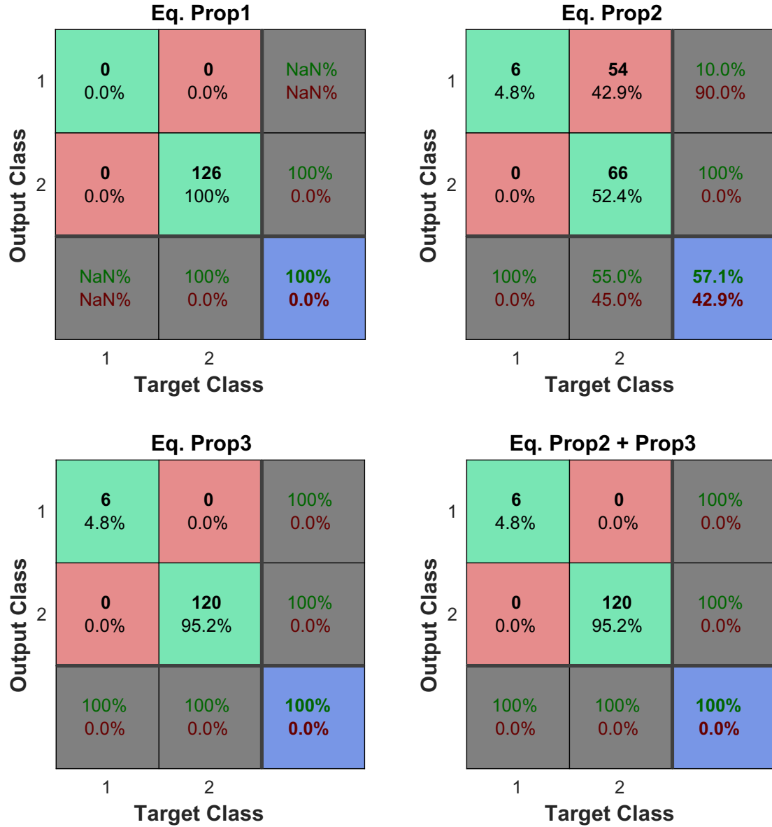
Figure 2.5: Confusion matrices obtained processing all the triplets in \mathcal{D}_{tr} . When considering Eq. Prop. 2.3.1, a sample is assigned to Class 1 if its markers and joint identify a prismatic transformation, while in the cases of Eq. Prop. 2.3.2 and 2.3.3 the elements in Class 1 identify revolute transformations.
