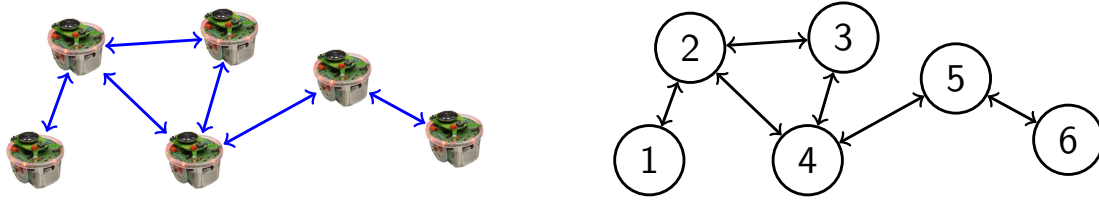
Figure 2.4: On the left a multi-agent system composed by N = 6 robots. As always, a blue arrow between two agents shows that these agents can communicate. The right part of the figure shows the underlying communication graph.
