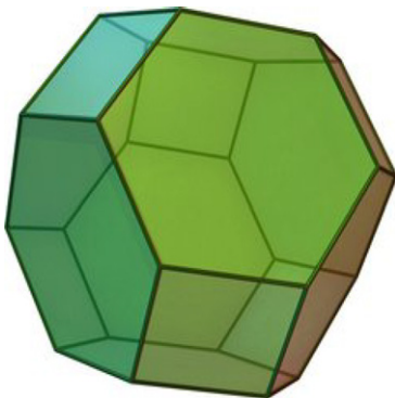
Fig. 25. A truncated octahedron has 14 faces; 8 are hexagonal and 6 are square. The length of the edges of hexagons and squares are the same. Figure is from [85].
