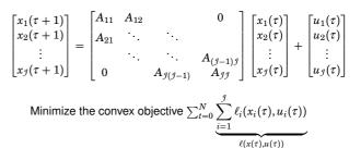
with convex constraints  $x_i(\tau) \in X_i$ ,  $u_i(\tau) \in U_i$  and  $x(0) = \bar{x}$ .
