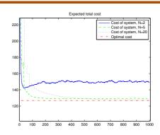
A distributed controller with 100 agents, using only local data. Fewer gradient iterations gives faster convergence, but worse stationary performance.
