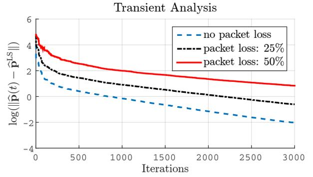
Fig. 4: Comparison between the a-GL solution and the optimal centralized LS solution, for different percentages of packet losses.
