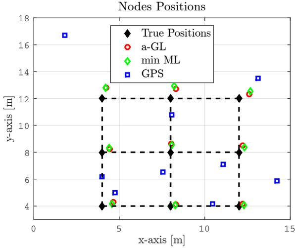
Fig. 1: Absolute positions for a formation of  $N = 9$  robots,  $\sigma_r = 0.1$  [m] and  $\sigma_\delta = 0.03$  [rad]. The black dashed line highlights the shape of the real formation as well as the communication graph.
