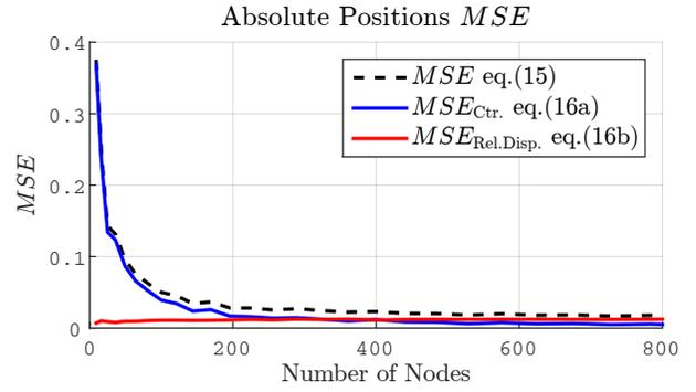
Fig. 2: Absolute positions  $MSE$ , computed via Monte Carlo simulations, as function of  $N$  for  $\sigma_r = 0.1$  [m] and  $\sigma_\delta = 0.03$  [rad].
