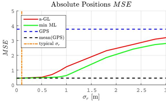
Fig. 3: Absolute positions  $MSE$ , computed via Monte Carlo simulations, as function of  $\sigma_r$  ( $\sigma_\delta = \text{atan2}(\sigma_r, \frac{4}{3})$ ) for  $N = 9$ . The dark orange vertical dashed-dotted line highlights the behavior corresponding to  $\sigma_r = 0.1$  [m].
