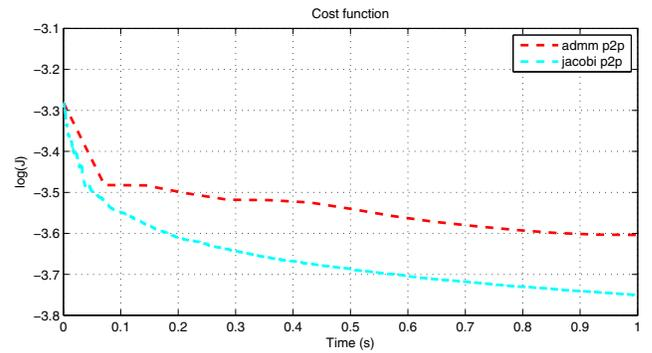
Fig. 3. Behavior of the error norm  $\|\hat{u}(t) - u^*\|$  for both the ADMM and the Jacobi-like estimation algorithm, in the case of a peer-to-peer architecture, as function of time. The norm of the error has been plotted in logarithmic scale.
