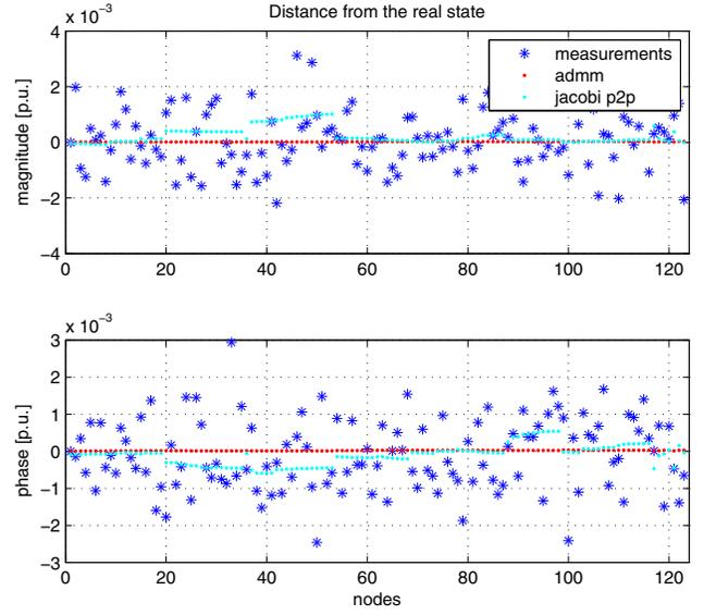
Fig. 1. Residual error at the steady state of the Admm algorithm (red) and of the Jacobi-like algorithm (blue), in the case of a peer-to-peer architecture, compared to the raw measurements.
