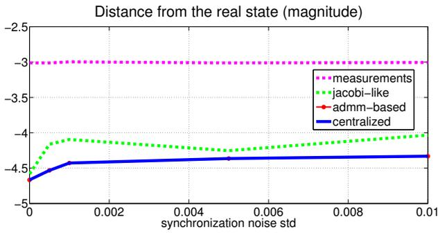
Fig. 2. Comparison of the norm of the magnitude estimation error for different values of the standard deviation  $\sigma_{\text{sync}}$ . Both algorithms have been reported, together with the raw measurements and the optimal centralized estimate (which corresponds to the estimate generated by the ADMM algorithm). The plot represents the average of 1000 trials, and the norm of the error has been plotted in logarithmic scale.
