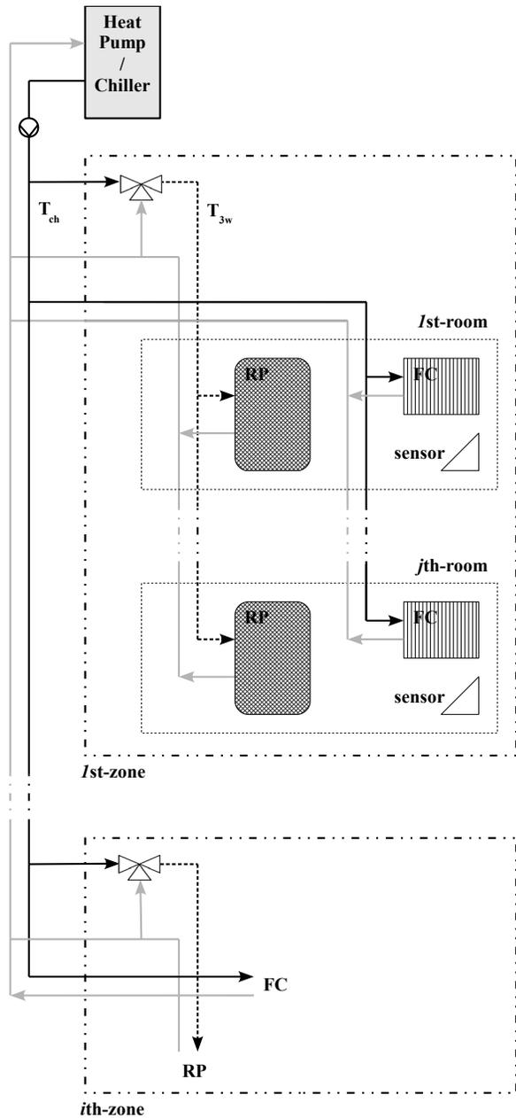
Fig. 1. Multiple zone radiant heating/cooling system: chiller, radiant panels (RP), fan coils (FC) and hygrothermal sensors.
