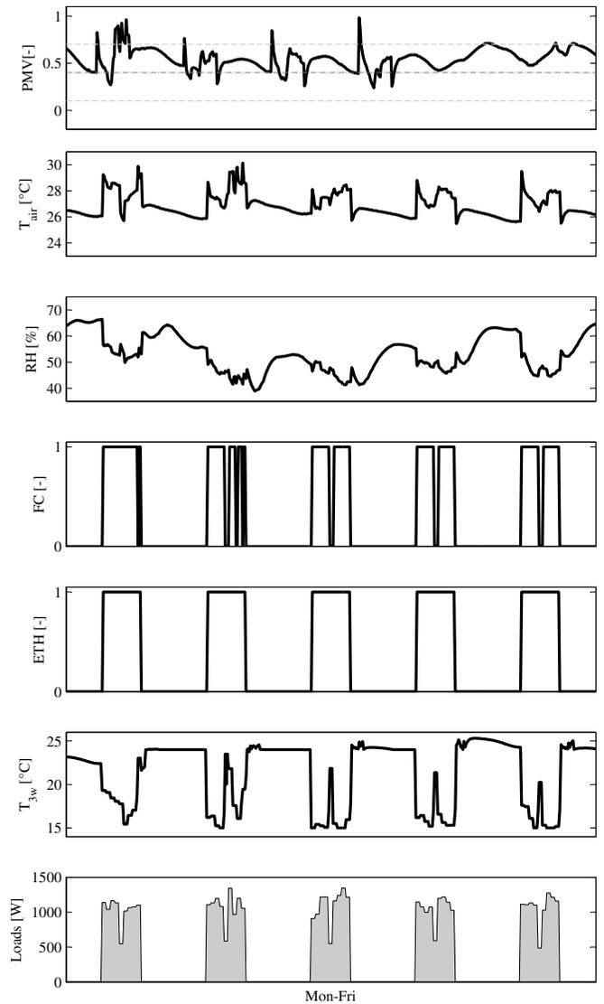
Fig. 3. *Comfortstat*, cooling mode (3rd Week of July, Mon-Fri): PMV,  $T_{air}$ , RH, FC operating time, ETH opening time,  $T_{3w}$  and internal loads.
