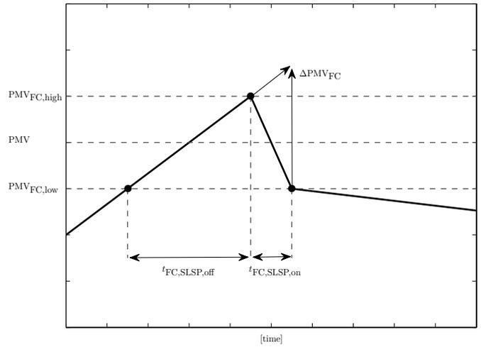
Fig. 2. Fan-coil: sensible load supporting period.
