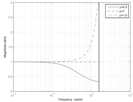
Fig. 5. Complementary Sensitivity Function  $|\eta|$  with  $\mu = 0.5, 1$  and  $1.5$
