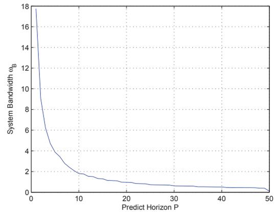
Fig. 7. Relations between Prediction Horizon  $P$  and System Bandwidth  $\omega_B$ . The System is  $G(s) = \frac{1}{0.5s+1}$
