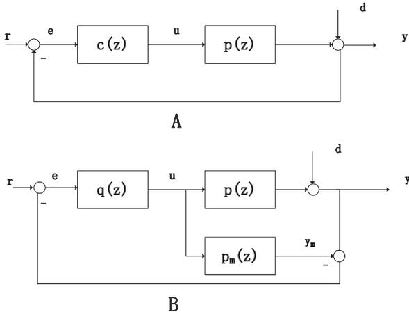
Fig. 1. General and IMC Block Diagram of Feedback Control System
