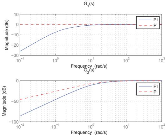
Fig. 2. Sensitivity Function with PI & P Controllers
