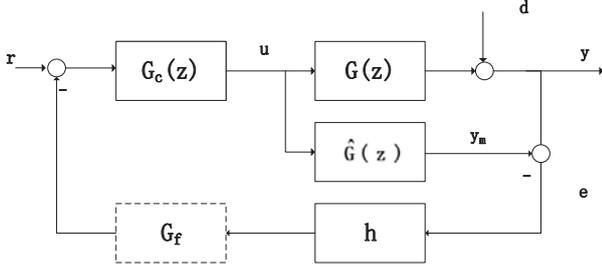
Fig. 3. DMC Block Diagram in IMC structure
