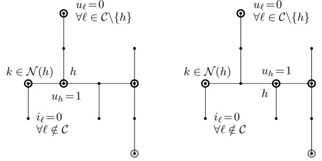
Fig. 4. A representation of how the elements  $G_{kh}$  are defined. Notice that in the configuration of the left panel, as the paths from  $h$  to its neighbors  $k \in \mathcal{N}(h)$  do not share any edge, the gains  $G_{kh}$  corresponds to the path admittances  $1/Z_{kh}$ .
