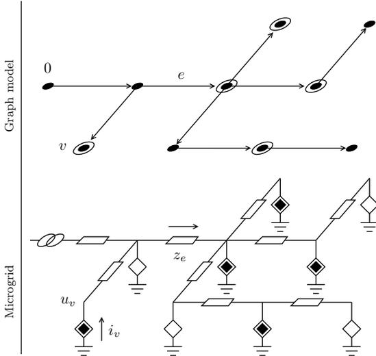
Fig. 1. The lower panel is a circuit representation of a microgrid, while the upper panel is the corresponding graph model. Black diamonds (below) and circled nodes (above) correspond to microgenerators connected to the microgrid. Node 0 corresponds to the point where the microgrid connects to the utility (PCC). The other nodes are the microgrid loads.
