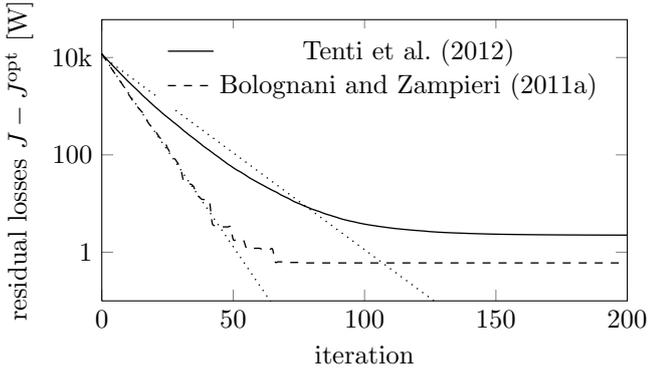
Fig. 5. The algorithm behavior (averaged over 1000 realizations), compared to the algorithm proposed in Bolognani and Zampieri (2011a). The dotted rays represent the corresponding analytic bounds on the rate of convergence.
