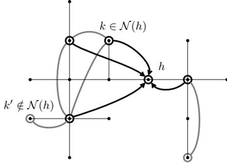
Fig. 3. The proposed communication architecture. The thick lines are the available communication links between the compensators (the circled nodes). Each node  $h$  is capable of collecting data messages only from the *neighbor compensators*.
