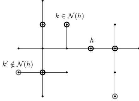
Fig. 2. An example of neighbor compensators. Circled nodes (both gray and black) are compensators. Nodes circled in black belong to the set  $\mathcal{N}(h) \subset \mathcal{C}_0$ . Node circled in gray are compensators which do not belong to the set of neighbors of  $h$ . For each compensator  $k \in \mathcal{N}(h)$ , the path that connects  $h$  to  $k$  does not include any other compensator besides  $h$  and  $k$  themselves.
