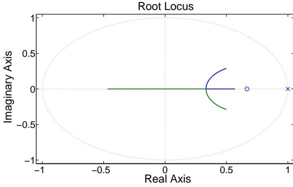
Fig. 1. Root locus of  $(z - 1)^2 + \lambda(z - 1 + \alpha) = 0$  for  $\alpha = 1/3$  as a function of  $\lambda \in [\lambda_2, \lambda_N]$ .
