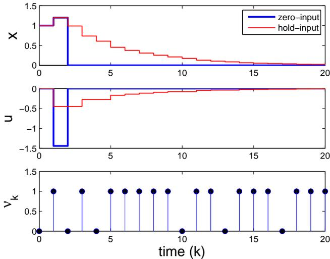
Fig. 3. A specific realization for  $A = 1.2$ ,  $x_0 = 1$ ,  $\bar{\nu} = 0.5$  under optimal zero-input control,  $l_z^* = -a = -1.2$  and optimal hold-input control,  $l_h^* = -(1 - \bar{\nu})a/(1 + \bar{\nu}a) = -0.375$ .
