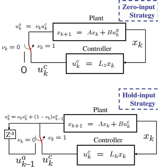
Fig. 1. Compensation approaches for actuators with no computational resources when a control packet is lost: zero-input approach  $u_k^a = 0$  (top) and hold-input approach  $u_k^a = u_{k-1}^a$  (bottom).
