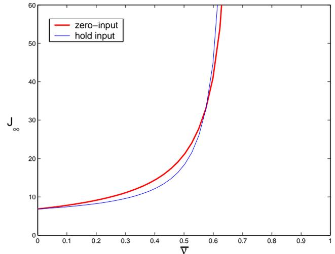
Fig. 5. Minimum cost  $J_\infty$  for  $A = 1.2$ ,  $B = W = x_0 = 1$ ,  $U = 10$  under zero-input and hold-input control architectures.
