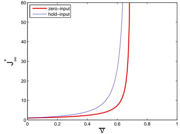
Fig. 2. Minimum cost  $J_\infty$  for  $A = 1.2$ ,  $B = W = x_0 = 1$ ,  $U = 0$  under zero-input and hold-input control architectures. The critical loss probability for this systems is  $\nu_c = 1/1.2^2 = 0.69$ .
