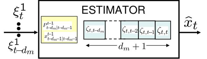
Fig. 5. Memory data structure required at the base station for the measurement fusion strategy.
