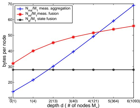
Fig. 7. Average number of bytes transmitted per node per time step as a function of the tree depth  $d$ . On the  $x$ -axis inside the round parentheses there are also indicated the corresponding total number of sensor nodes in the network.
