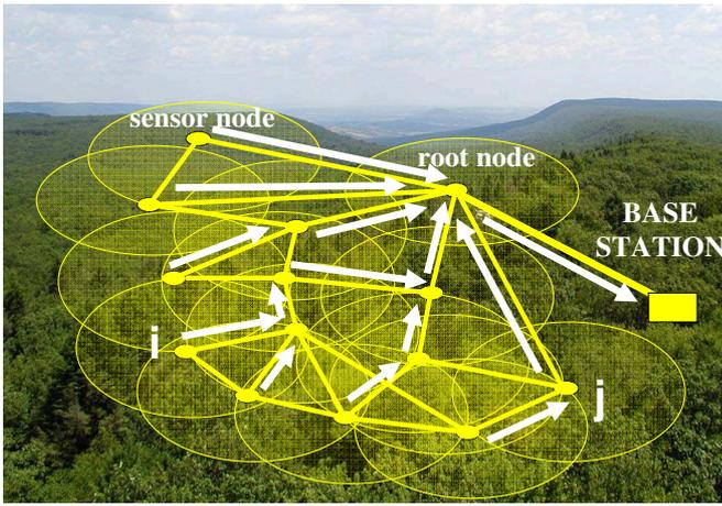
Fig. 1. Pictorial representation of Wireless Sensor Network for environment monitoring. The small dots indicate the location of the sensing nodes, the shaded circles indicate the sensing regions and the segments the communication links. White arrows represent the tree-based routing paths from the sensor nodes to the root sensor node and to the base station.
