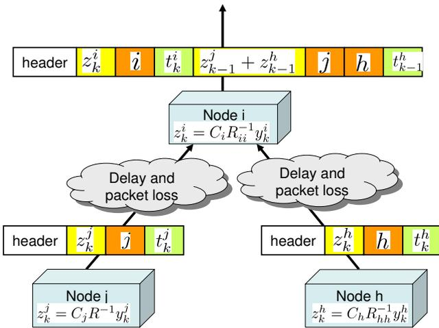
Fig. 4. Data packet structure transmitted by each sensor node for the measurement fusion strategy.
