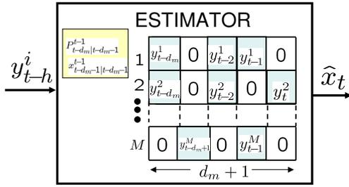
Fig. 3. Memory data structure required at the base station for the measurement aggregation strategy.
