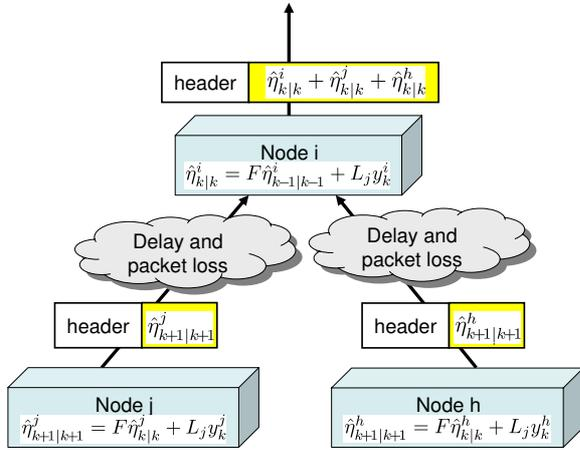
Fig. 6. Data packet structure transmitted by each sensor node for the partial state estimate fusion strategy.
