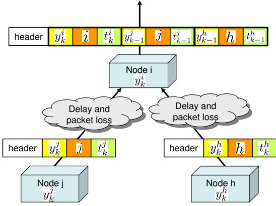
Fig. 2. Data packet structure transmitted by each sensor node for the measurement aggregation strategy.
