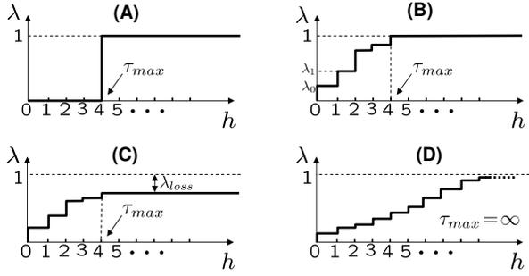
Fig. 3. Probability function of arrival process  $\lambda_h = \mathbb{P}[\tau_k \leq h]$  for different scenarios: deterministic packet arrival with fixed delay (A); bounded random packet delay with no packet loss (B); bounded random packet delay with packet loss (C); unbounded random packet delay with no packet loss (D).
