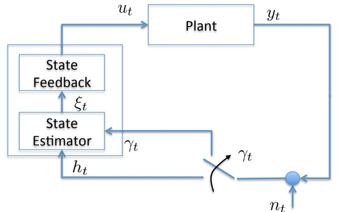
Fig. 2. NCS scheme for scalar output plants, where the plant decoder is given by the cascade of a linear state estimator and a state feedback
