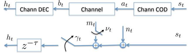
Fig. 2. Equivalent model of Channel COD/DEC using traditional codes
