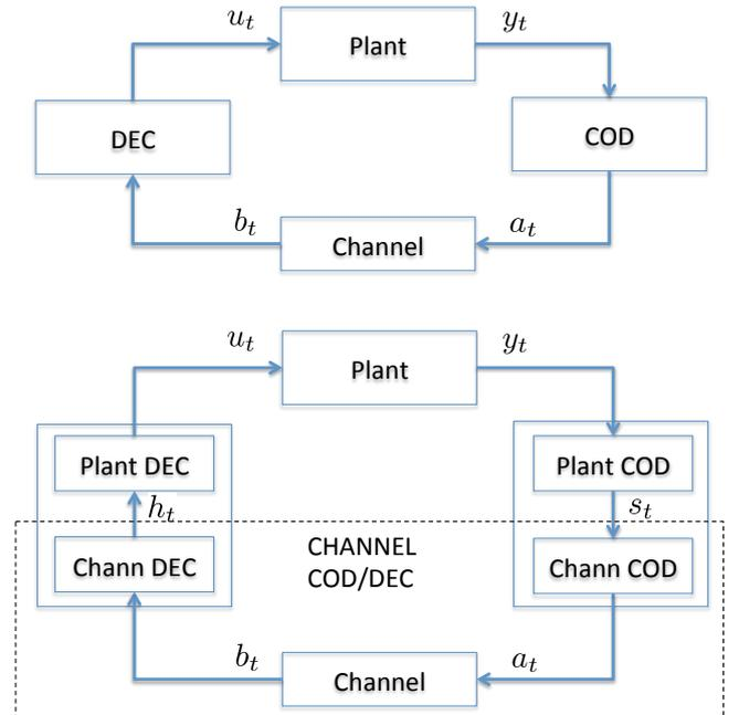
Fig. 1. Scheme of control system across a communication channel: general scheme (top), decoupled scheme (bottom).
