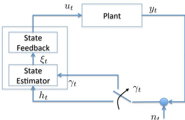
Fig. 4. Special scheme of Networked Control System for scalar output plants
