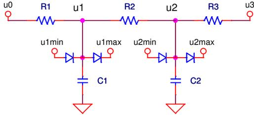
Fig. 5. Electric circuit with saturation constraints.
