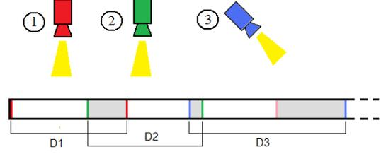
Fig. 1. Perimeter under surveillance. The physical coverage  $\{D_i\}$  of three cameras is shown, with some overlapping sections.
