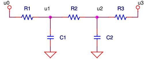
Fig. 4. Electric circuit analogy ( $N = 3$ ). Voltages  $\{u_i\}$  relate to the positions of the patrolling sections  $\{A_i\}$ .
