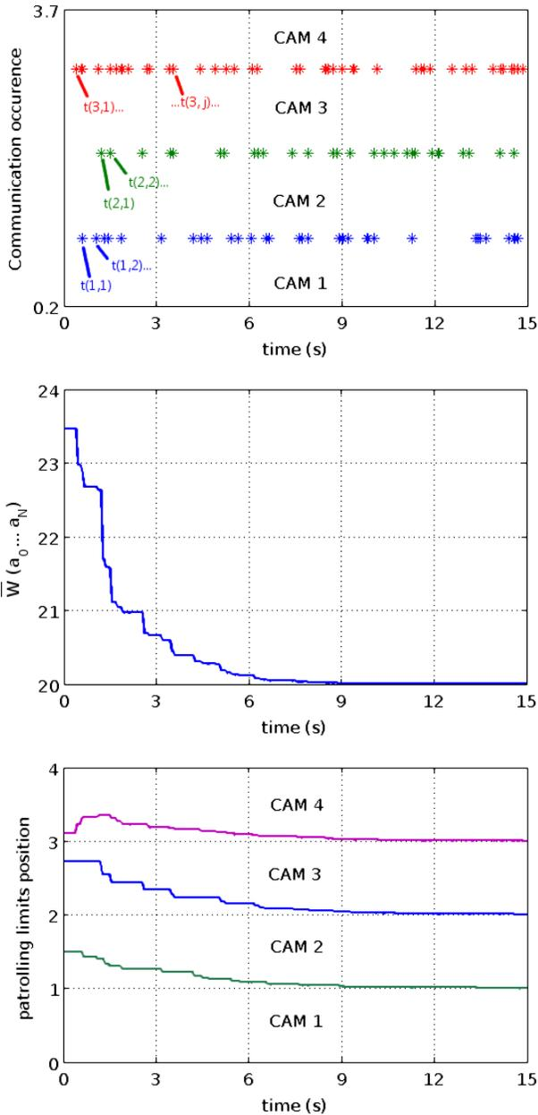
Fig. 6. Asynchronous communication pattern between cameras (*top*), and corresponding global Lyapunov-like function (*center*) and patrolling boundaries (*bottom*) for 4 cameras.
