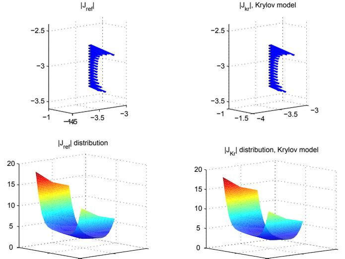
Fig. 4. Comparison between full model ( $n = 2773$ ) output and Krylov-reduced one with  $\tilde{n} = 30$ . Upper plots show the current density vector field  $\vec{J}$  through the section of the vertical structure, whereas the bottom figures show the amplitude  $|\vec{J}|$  above the section.
