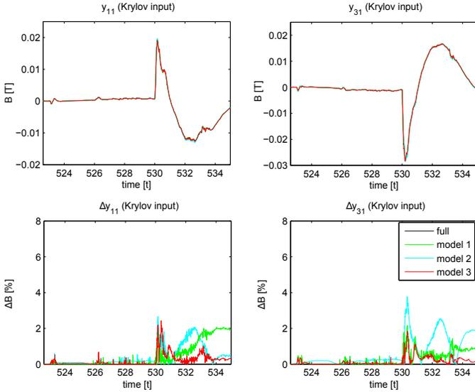
Fig. 3. Time evolution of two sample measurements output ( $m_{11}$  and  $m_{31}$ ) obtained using Krylov input algorithm, with the respective percentage errors.
