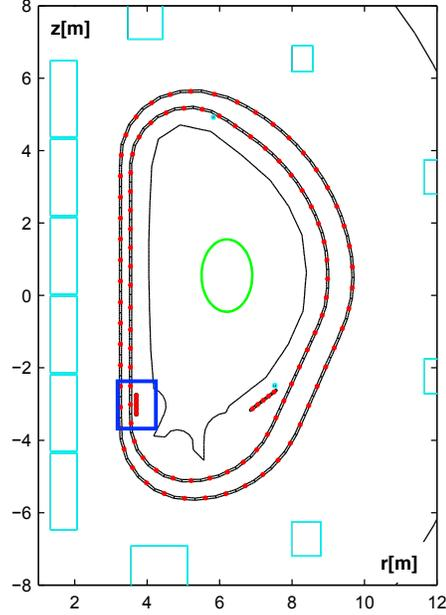
Fig. 1. ITER-like machine cross section and circuits representation.
