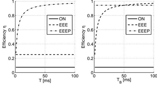
Fig. 3. Efficiency comparison for a specific trace (R1G #A1, Table III). On the left, the efficiencies of the strategies Always-On (ON), EEE and EEEP are compared vs the time window length  $T$  (with  $N_{th} = 15$ , which leads to  $\bar{T}_B \approx 1$ ms). On the right, the efficiencies are compared vs the mean burst unit duration  $\bar{T}_B$  (with  $T = 50$ ms).
