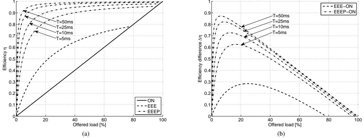
Fig. 4. Efficiency of the strategies vs offered load, for different window lengths  $T$ . (a) The dashed lines refer to the EEE and EEEP strategies; the solid line corresponds to the Always-On policy. (b) The dashed lines refer to the difference between the two energy efficient strategies and the Always-On policy.
