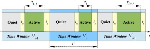
Fig. 2. EEEP strategy. Schematic drawing of operation.
