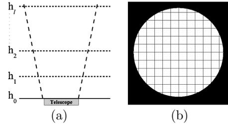
Fig. 2. (a) Atmospheric turbulence is modeled as a superposition of  $l$  layers. (b) Discrete domain  $\mathbb{L}$ .
