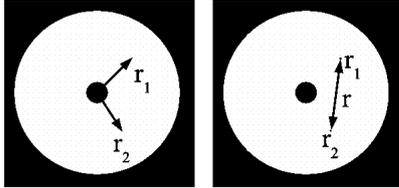
Fig. 1. Telescope image domain: Two points,  $r_1$  and  $r_2$ , separated by a distance  $r$  on the telescope aperture plane.
