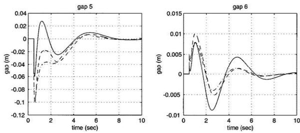
Fig. 5: Linear vs nonlinear simulations: gap behavior after application of a disturbance. Solid line: nonlinear simulation; dashed and dash-dotted lines: two different linear models.
