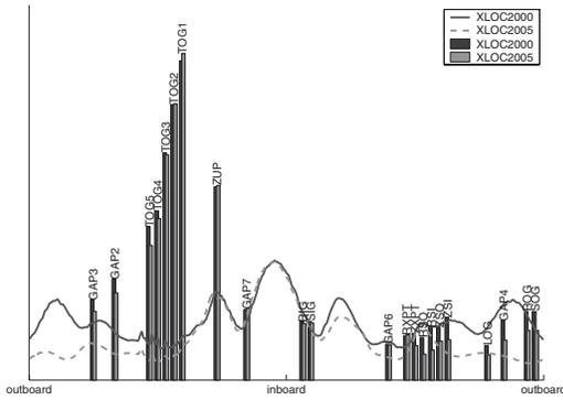
Fig. 4: Magnetic refurbishment. Error propagation on the magnetic field reconstruction and correspondence with the gap reconstruction provided by the real time code.
