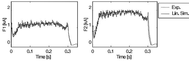
Fig. 7: RFX model. Validation with experimental data of the linear model of RFX derived from the nonlinear model implemented in MAXFEA.
