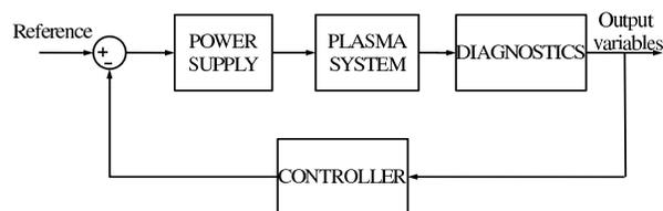
Fig. 1: Control Loop scheme. The open loop is the cascade of power supply, plasma-vessel system, and diagnostics.
