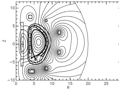
Fig. 2: MAXFEA Flux map. Example of output flux map provided by the code with reference to the ITER machine.
