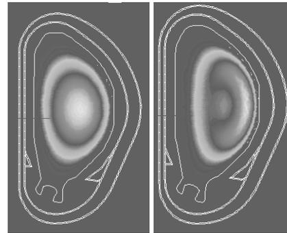
Fig. 6: Plasma current distribution for ITER equilibria. Nominal (left) and reverse shear (right) current profiles.
