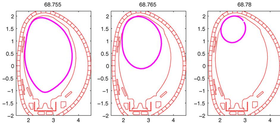
Fig. 6. Reconstruction of the evolution of the plasma shape during a disruption obtained using the CREATE model.
