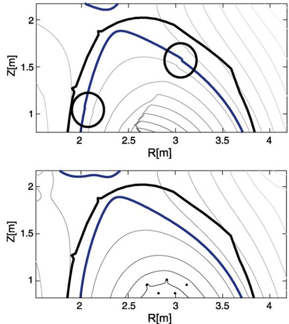
Fig. 5. Comparison between Taylor expansion model (left) and filamentary model (right) boundary reconstructions.
