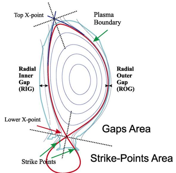
Fig. 3. Plasma geometry identification.  $x$ -Points top and lower, gaps, strike points are some of the objects identified by Felix.
