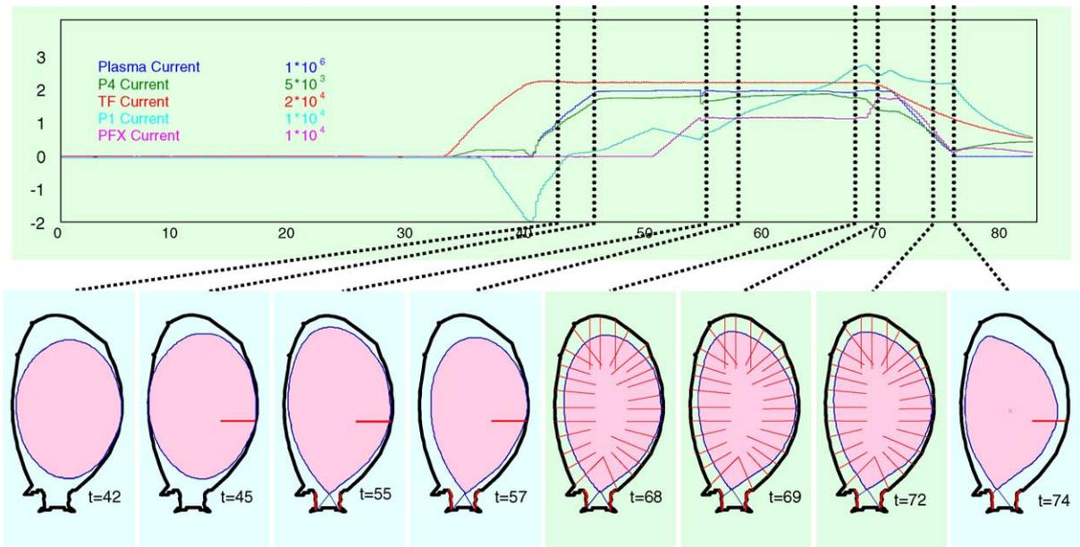
Fig. 3. JET pulse #61995. The XSC is activated in the time windows 68–72 s, and controls 32 gaps and 4 additional geometric descriptors representing the whole boundary shape. Before  $t = 68$  s, SC controls the circuit currents and the radial outer gap only.
