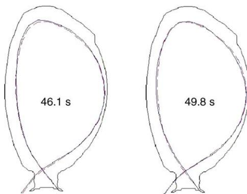
Fig. 5. JET pulse #62292, characterized by a wide ITB, in which the XSC has been used from 43.5 to 50 s. The desired shape (dashed line) is kept within a maximum error of 5 cm close to the upper and lower X-points in the presence of a wide  $\beta_{\text{pol}}$  excursion:  $\beta_{\text{pol}} = 1.6$ ,  $l_i = 0.8$ ,  $I_p = 1.53$  MA at time = 46.1 s;  $\beta_{\text{pol}} = 0.1$ ,  $l_i = 1.0$ ,  $I_p = 1.48$  MA at time = 49.8 s.
