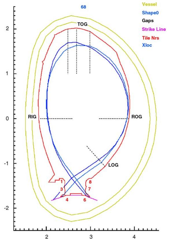
Fig. 2. Detail of the graphic window of JET XSC controller interface for the Session Leader, showing the gaps used by the old SC.
