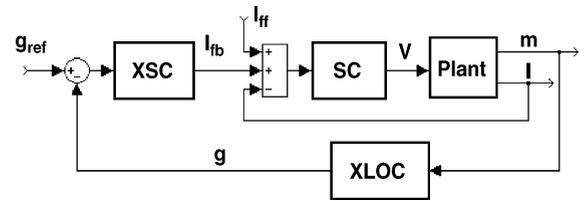
Fig. 1. JET XSC controller architecture.
